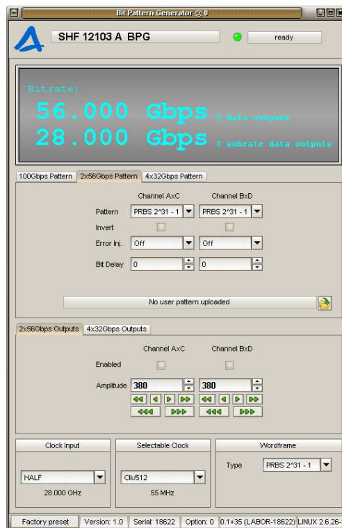
-Screenshot from the SHF BERT control software showing the SHF 12103 A window-
