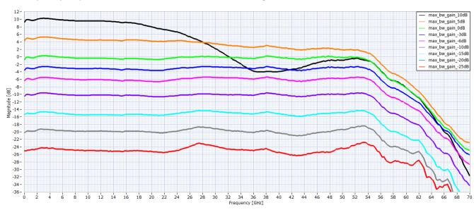
Frequency responses for a 3, 6, 9 and 12 dB slope @ 35 GHz
